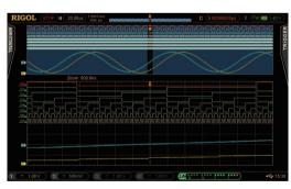
Deeper memory depth for the digital channels, serial bus triggering and decoding on digital channels
